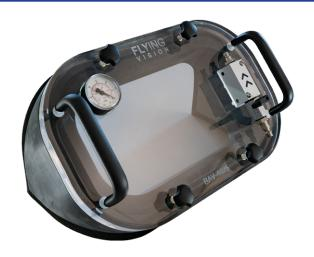
The BAV4O25IA is an NDT vacuum box for internal right angles, designed for leak testing 90° internal corner welds, such as inside storage tanks to inspect the shell-to-bottom joint, and also in all types of tanks and containers across various industrial sectors. Its interchangeable base offers great flexibility for inspecting different surfaces and weld configurations, enabling rapid leak detection.
