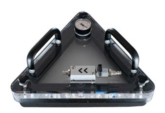
The BAV4OIC is an NDT vacuum box designed for internal right-angle corners, tailored for leak testing 90° internal corner welds, such as inside mechanically welded assemblies, tanks, containers, on the corners of flat roofs, terrace roofs with waterproofing membranes, and more. Its interchangeable base offers great flexibility for inspecting different surfaces and weld configurations, enabling rapid leak detection.
